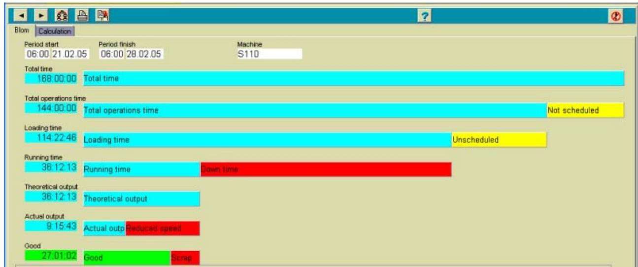
Figure 1: BLOM diagram showing the elements of OEE
