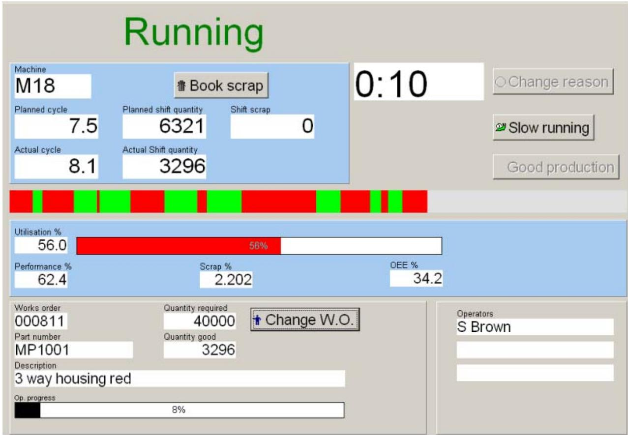
Figure 2: Monitoring PC machine status screen
